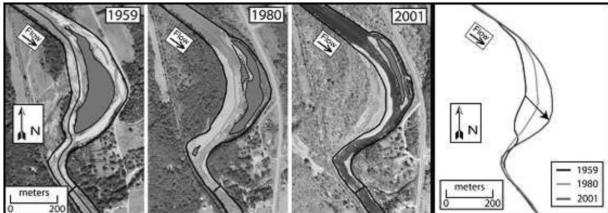
Figure 23. Changes in meander geometry at Beechford. From Miller, 2009.
